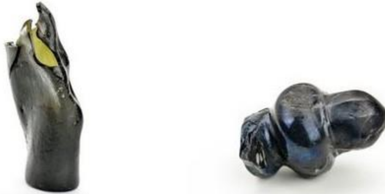
Left: Heat and pressure softened and twisted this champagne bottle. Right: A glass doorknob melted on one side, just as trees observed by Hovey were scorched on one side and, on the other, "green as if no eruption had occurred."
